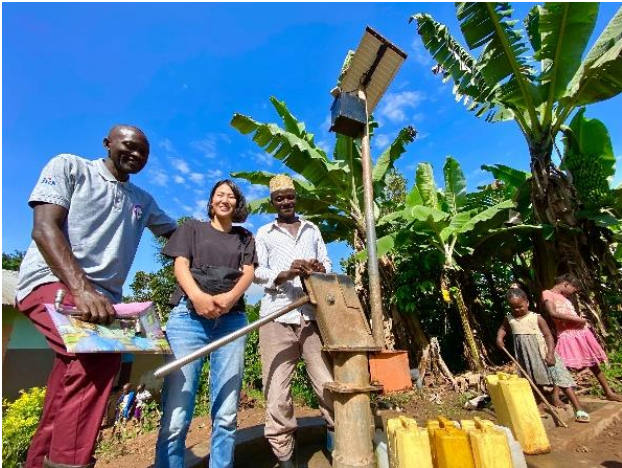
Automated charge collection system with mobile money for handpump Source: Sunda Technogy Global
